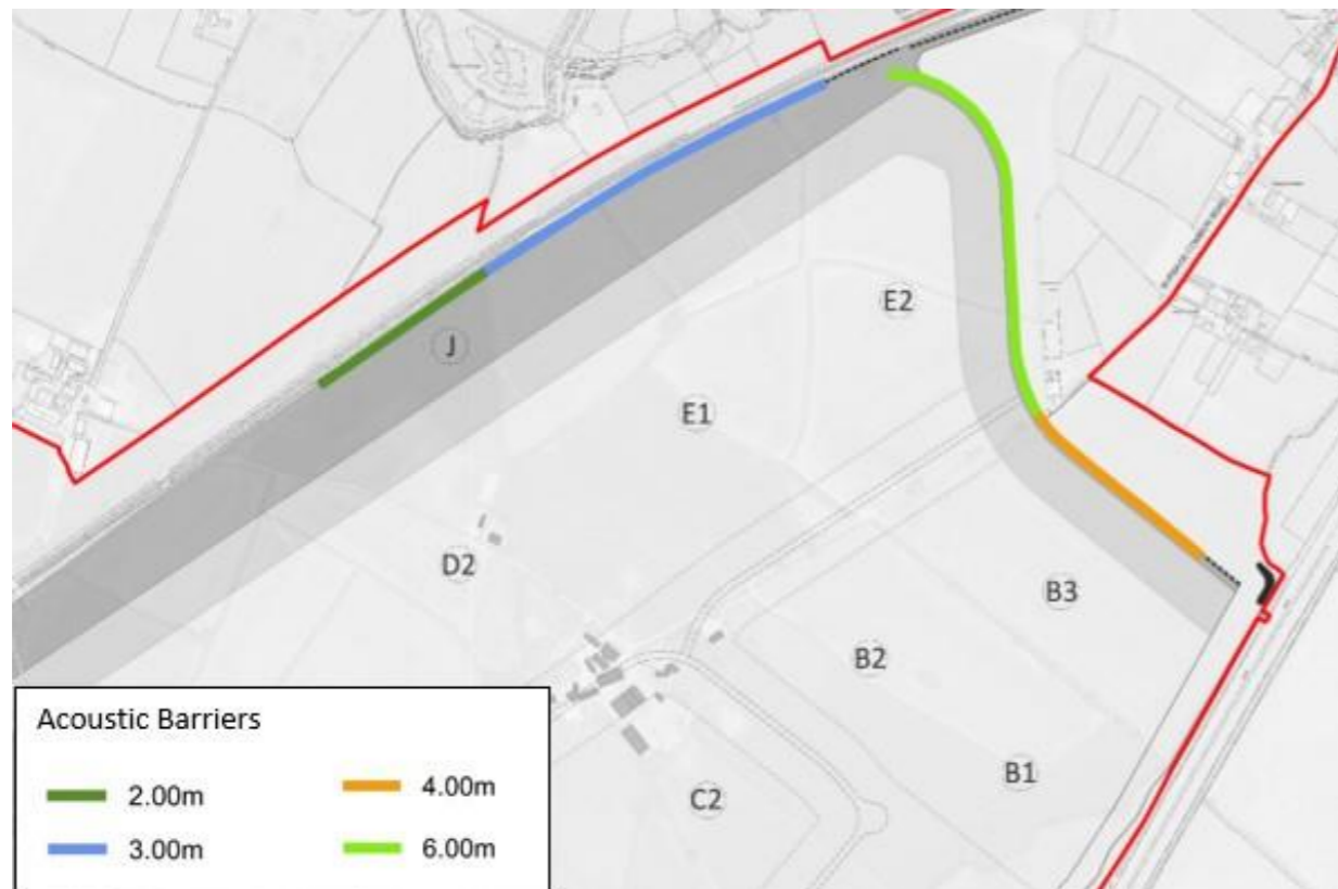
Fig. 612 Proposed Noise Barriers to north west of Railport and to the north east of head shunt (Document Reference 6.3.10.10, APP-279)
