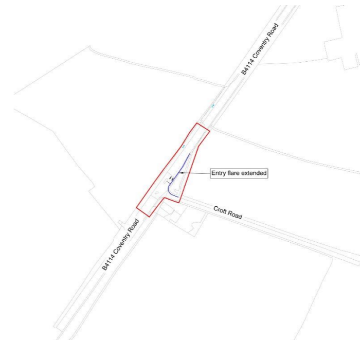
Fig 534. Proposed Works to Coventry Road / Croft Road junction east of Croft (Document Reference 6.3.3.3, APP-232)
